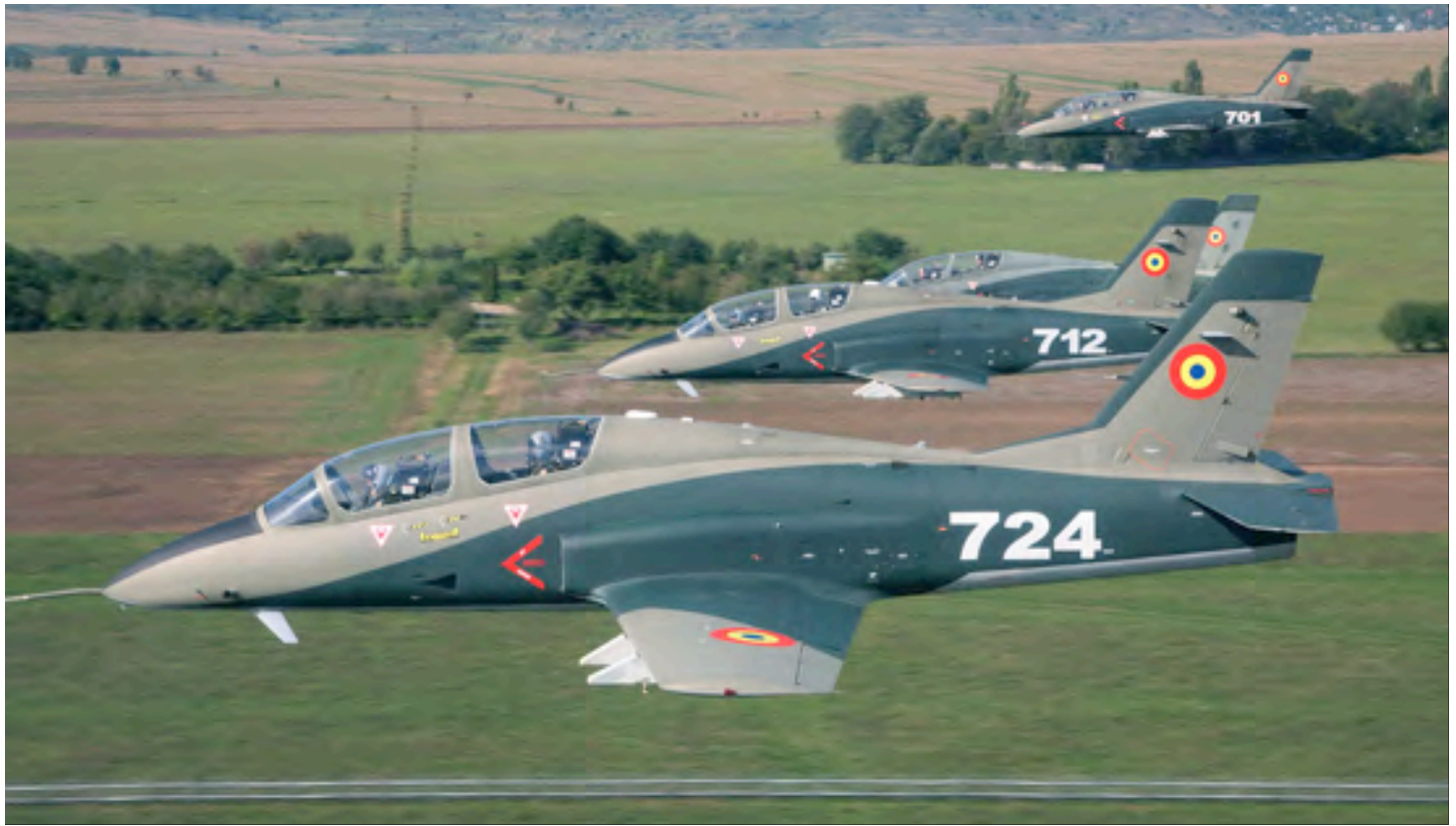
Above: The IAR-99 fulfils basic and advanced training needs for the Fortele Aeriene Romane. The two aircraft in the foreground are IAR-99C Soims, readily distinguished from the Standard by the radar warning receiver antennas on the tail and forward fuselage.
