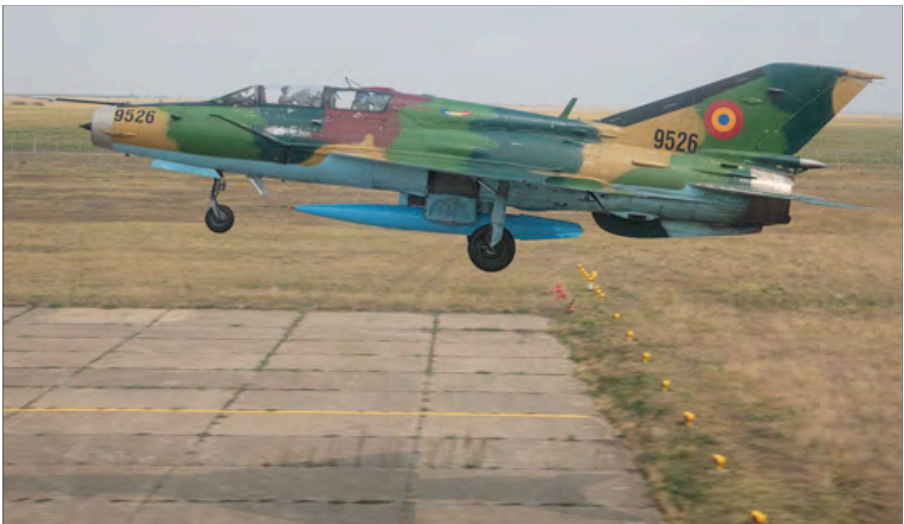
Above: The LanceR C modification is arguably the most advanced MiG-21 version flying. Its Elta multi-mode radar gives it good capability in the air defence role, while the DASH helmet sight allows high off-boresight missile shots.
