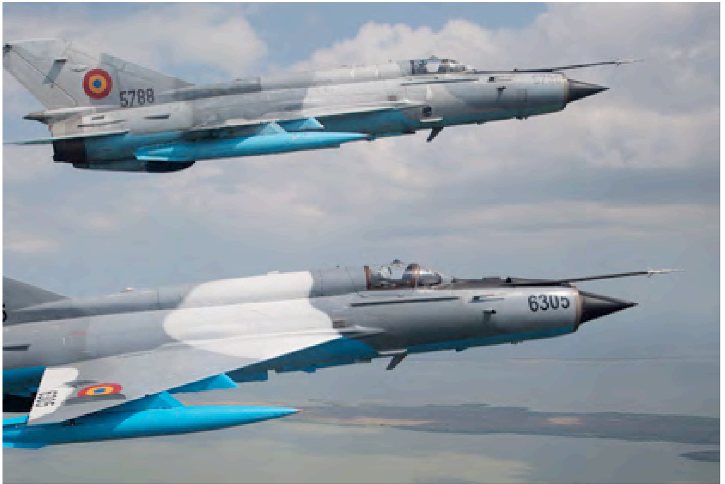
Above: The LanceR C modification is arguably the most advanced MiG-21 version flying. Its Elta multi-mode radar gives it good capability in the air defence role, while the DASH helmet sight allows high off-boresight missile shots.
