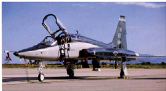
The 586th's AT-38s have an equipment bay in the spine that can house various test instruments. This example carries an unusual test fixture.
