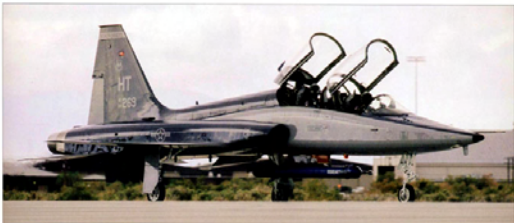
Above: Many of the test fixtures are carried on the centerline pylon of the AT-38B, but in this case the aircraft carries an ALQ-167 'Squeaky' programmable ECM pod. Jamming is required for many of the tests performed by the 580th FTTS. Inflight controls for centerline stores can be fitted in the rear cockpit.
