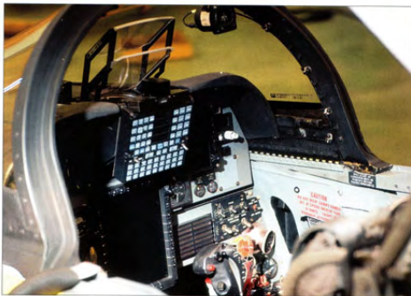
Having flown in the F-5M – with its HUD, MFD and large UFCP – the cockpit of the Eurofighter will not seem so unfamiliar. Furthermore, the avionics and datalink system allows the replication of radar functions in the F-5M without the expensive installation of a radar.
