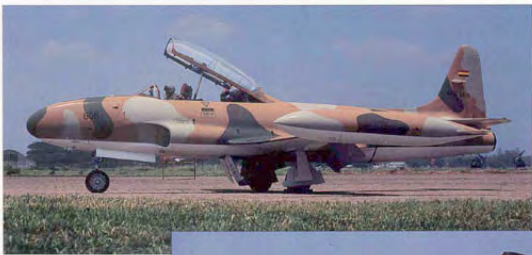
Following refit (including glass cockpit) by Kelowna Flightcraft in Canada, the Bolivian Lockheed T-33s are now known as T-33-2000s. This was the first aircraft to be returned to Bolivia, arriving with two others at El Alto air base on 8 August 2003. It served as the test airframe for the upgrade, and underwent extensive ground and air testing before its redelivery.
