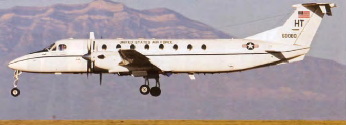
left: The 586th FLT's Beech C-12J (86-0080) is the sole example of this Beech 1900 derivative in US military test service. (Don Logan)
