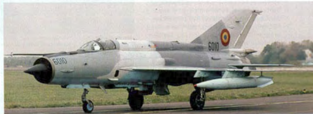
Lancer 6010 (a further example can be seen behind) taxis past, carrying a pair of fuel tanks under the wings.
