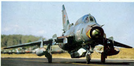
ABOVE: The Bulgarians provided a recce capability by sending a single Jambol/Bezmer based Su-22M4 equipped with the KKR recce/ELINT pod on the centre line stores station. MARIN SAF/WAS
