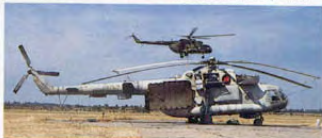
Below: Mi-17PP Hip-K serialised 707 is a Bakony Combat Helicopter Regiment helicopter which did not participate in the exercise. It is normally used for ECM communications jamming — hence the large 32-element panel on the side.
